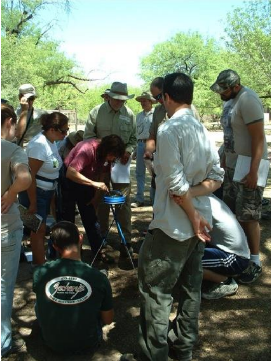
Figure 6: Volunteers Learning to Use a Solar Pathfinder at the Springs Inventory Protocols Training
